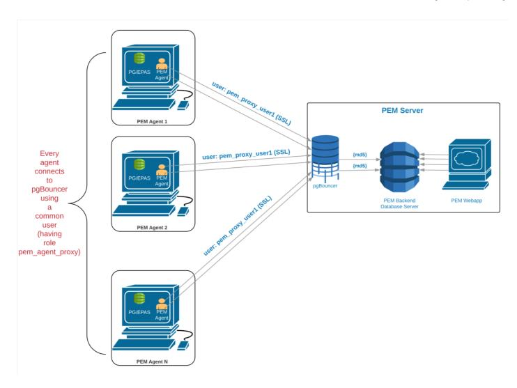
We recommend using PgBouncer version 1.9.0 or later as the connection pooler. Versions 1.9.0 or later support cert authentication. PEM agents can connect to pgBouncer using SSL certificates.
